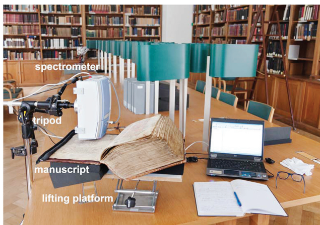
Figure 5. The FTIR instrument ALPHA of Bruker, Germany during the measurement in the Austrian National Library in Vienna
