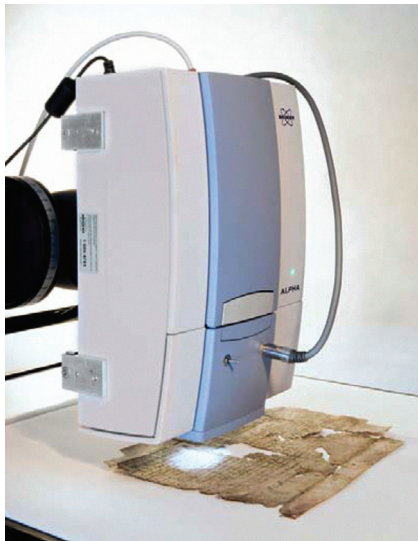
Figure 9. FTIR analysis of ink on parchment (left) and area of analysis (red), seen by the CCD camera of the instrument (right)
